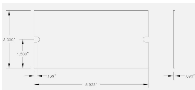
Transig PN 9701, Remote CT Isolation Unit Mounting Dimensions and Component Layout
